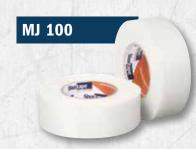
Open weave fiberglass mesh tape used for reinforcing joints, seams and connections when paint-on mastic is used in HVAC applications, and can also be applied to drywall seams before the application of joint compound, MI 100 drywall tape is self-adhering and offers superior strength compared to paper.
