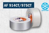
Linered cold temperature aluminum foil tape for joining and sealing aluminum-backed and fibrous insulation and metal ductwork, and to repair metal and sheet metal. Both AF 914CT and AF 975CT deliver an airtight seal in temperatures ranging from -20 F to 260 F. AF 914CT is 1.5 mil: AF 975CT is 2.0 mil.
